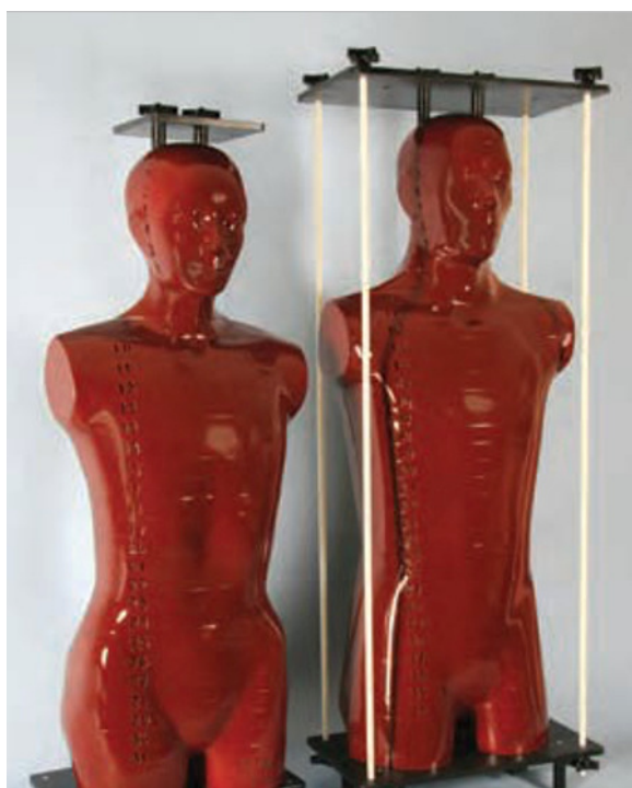
Figura 2.16 – Fantomas Alderson Radiation Therapy (ART) masculino e feminino. Fonte: (RADIOLOGY SUPPORT DEVICES, 2021)
