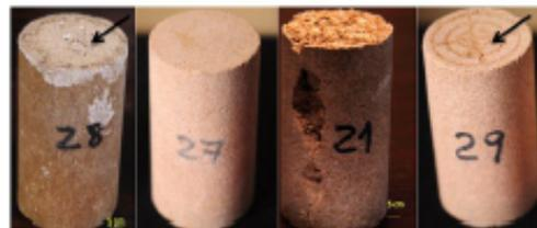
Figure 1: Indiana carbonate core samples used in the acidizing procedure performed with EDTA.
